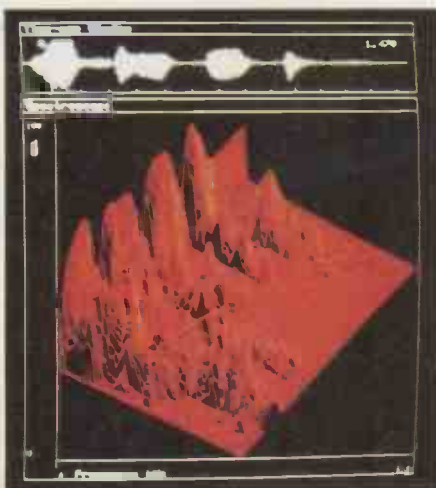
A 3D representation of speech patterns, part of the project to develop voice-activated word processing.
